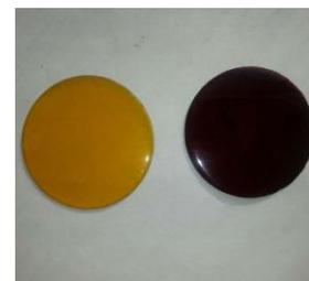
Fig.2 Samples that before and after the thermal aging
